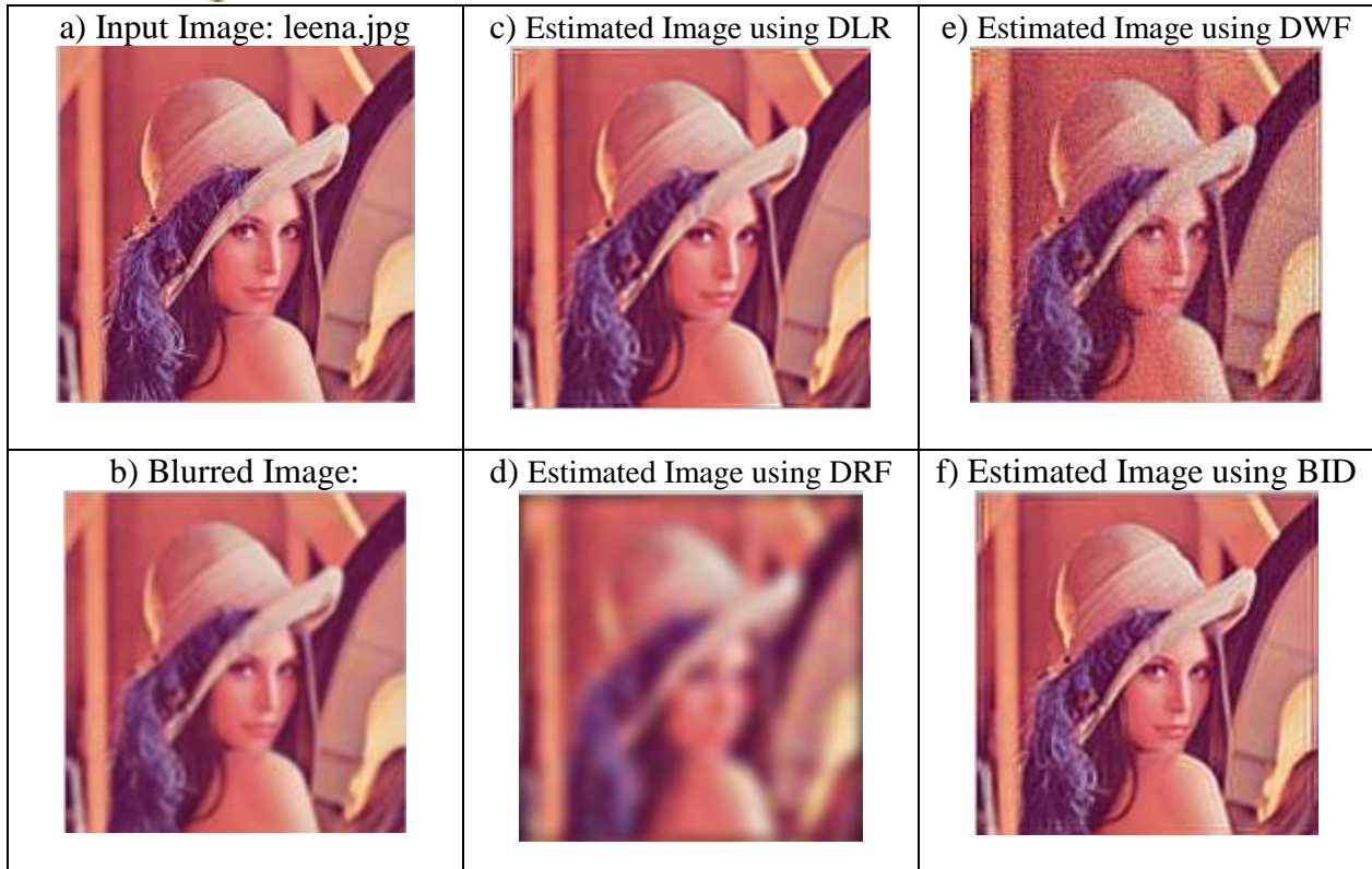
Fig. 5: Restoration Results for leena.jpg (256 x 256) blurred using a Gaussian Blur of size=5 and standard deviation=5
